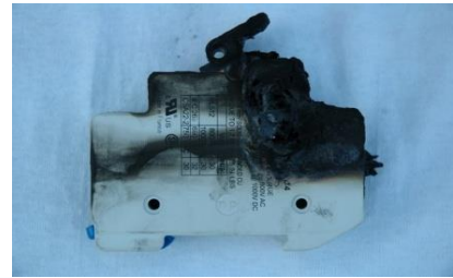
Fuseholder opened under load!!
