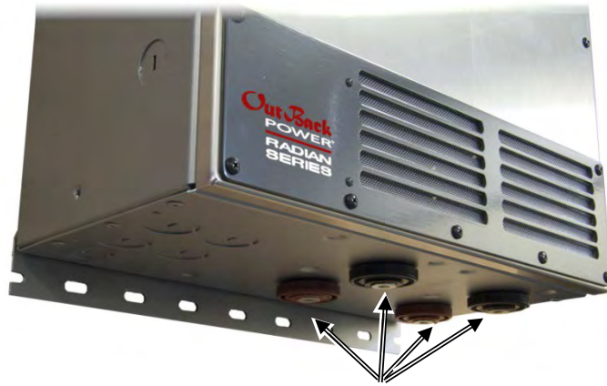
DC TERMINALS: Connects to the battery cables and DC system. There are two DC positive and two DC negative terminals. Each DC positive terminal requires separate cables and separate overcurrent protection. See page 20 for instructions.
